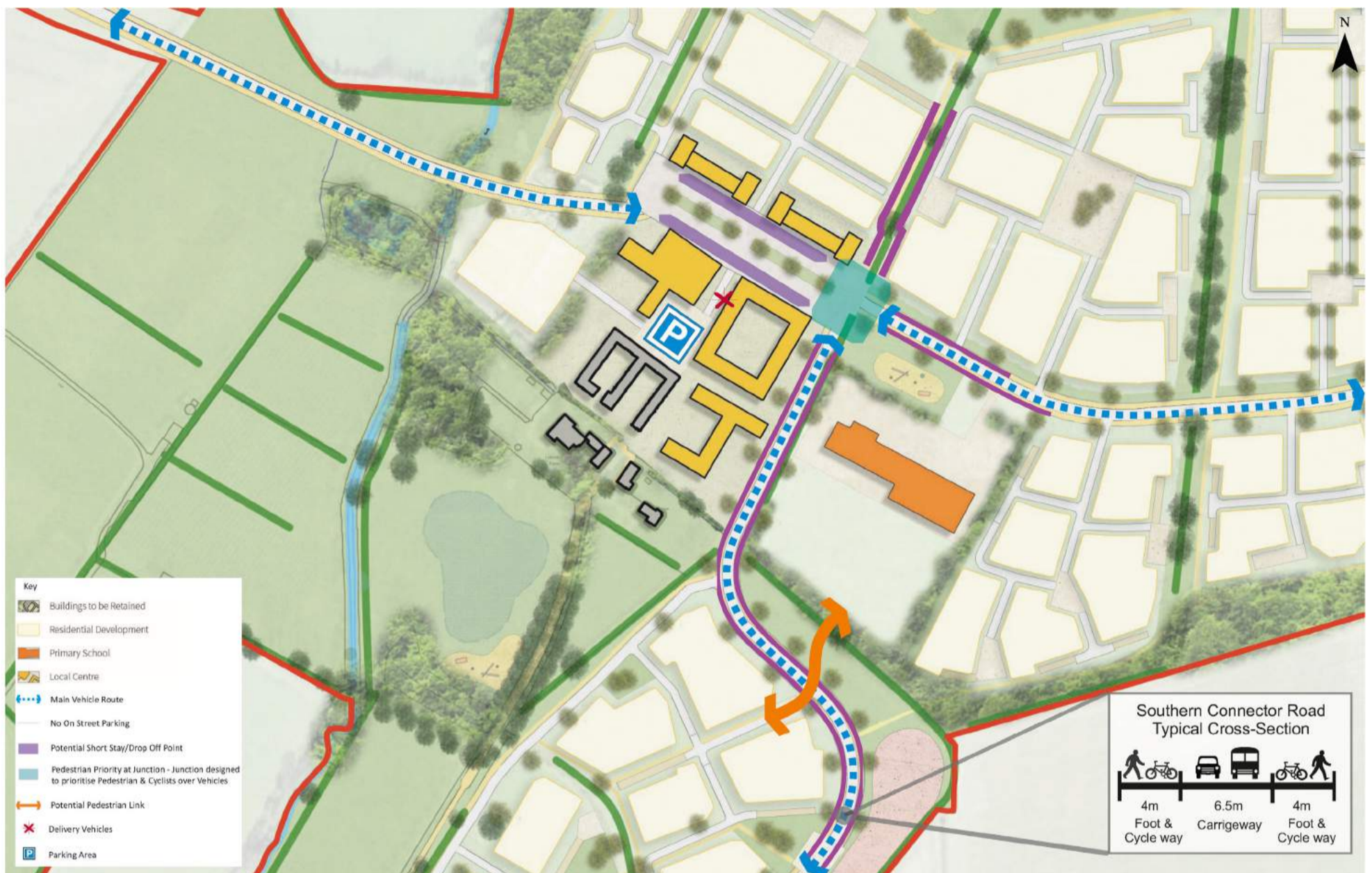
FIGURE 5.7 PRINCIPLES OF MOVEMENT AROUND LOCAL CENTRE PLAN (PLAN PRODUCED BY PETER BRETT ASSOCIATES)
