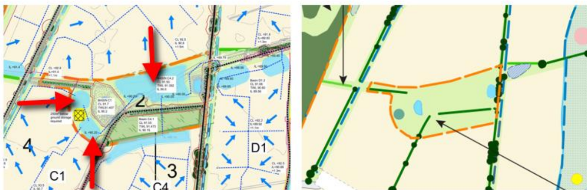
Figure 8.1: Proposed changes to Drainage Strategy and FRA Addendum in area of central Biodiversity Zone. Left image shows snapshot of proposed changes (DWG. 22006-HYD-P0-XX-DR-C-2222 P03). Right image shows snapshot of approved parameter plan (DWG. DWG. PL1461.1-PLA-00-XXDR-U-0005 P04).
