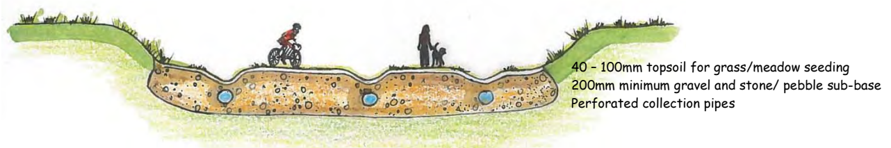
Figure 38 Swales in public open space
