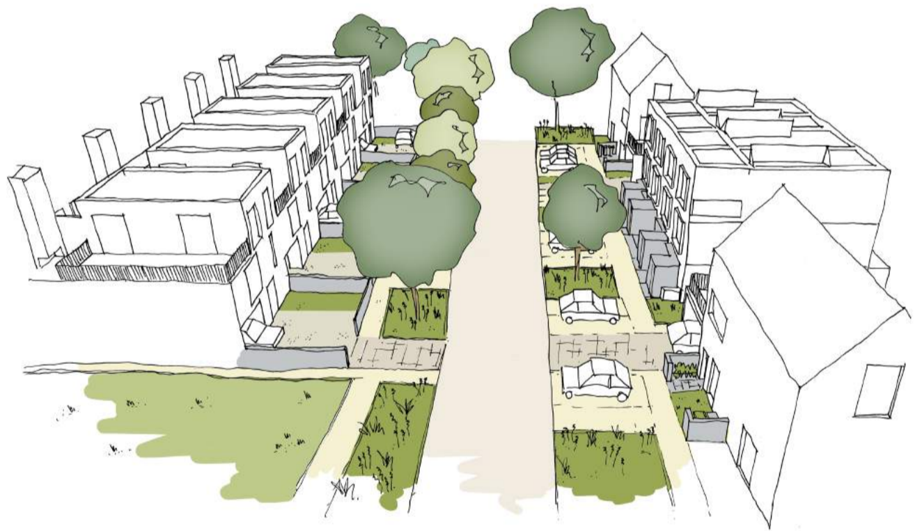
SKETCH SHOWS TREES AND PLANTING INTEGRATED WITHIN THE STREET TO REDUCE THE IMPACT OF THE CAR
